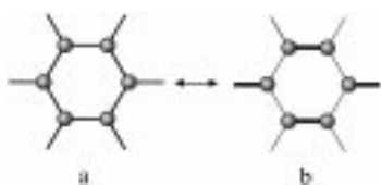
Scheme 1. Limiting structures of the phonon in a \text{B}_2^{2-} sheet in \text{MgB}_2 which is relevant for the occurrence of superconductivity: a) “benzoid” with equal B-B distances and b) “quinoid” with short (bold) and long B-B distances.
