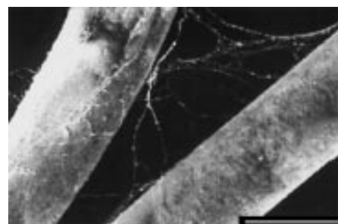
Figure 6. Polystyrene fibers collected on a bent copper wire (magnification 33\times ) and subsequently coated with a thin layer of polypyrrole by in situ deposition from aqueous solution. Scale bar: 1 mm.
