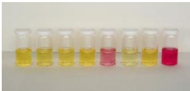
Figure 1. Color changes induced on 1 ( 1.0 \times 10^{-4} M) at pH 6 in the presence of the following anions in dioxane/water (70/30 v/v): from left to right: no anion, bromide, chloride, phosphate, sulfate, GMP, ADP, and ATP.
