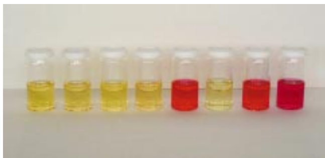
Figure 3. Color changes induced on 2 ( 1.0 \times 10^{-4} M) at pH 6 in the presence of the following anions in dioxane/water (70/30 v/v): from left to right: no anion, bromide, chloride, phosphate, sulfate, GMP, ADP, and ATP.
